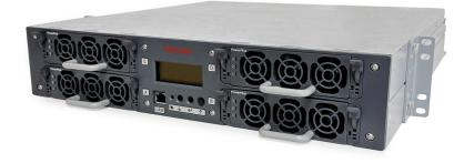
The PowerPlus System is a power conversion system for up to 12 independent high power DC circuits, with a maximum load current of 50A each, feeding new generation high-power RRH units.
