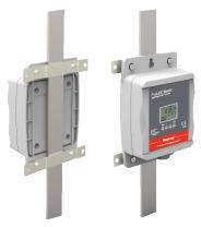
ProLEC Basic is a basic lightning current sensor that detects and logs lightning discharges flowing through the down-conductor. It is capable of measuring and withstanding currents up to 100 kA (10/350 μs).
