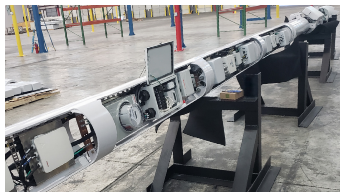
Small cell poles, like these at one of Raycap's three manufacturing facilities, contain and conceal complete small cell sites.
