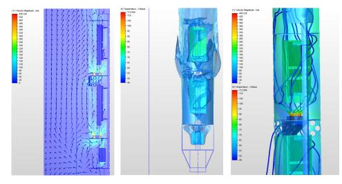
Simulation results are confirmed with physical testing, often in partnership with **Original Equipment Manufacturers** (OEMs). This testing is performed both on-site and by partnering with world-class third-party test facilities to employ thermal chambers to simulate high ambient temperature conditions. When weather is uncooperative, solar load can be simulated in the test environment by high-powered metal-halide lamps.
