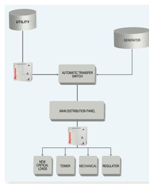
Figure 1: A typical airport installation can protect critical electronics from devastating surges in voltage.
