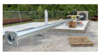
Pole Mounted to Test Fixture (3UN Orientation)
