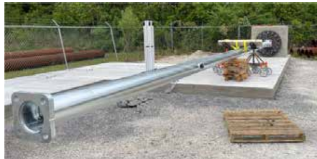
Pole Mounted to Test Fixture (3UN Orientation)
