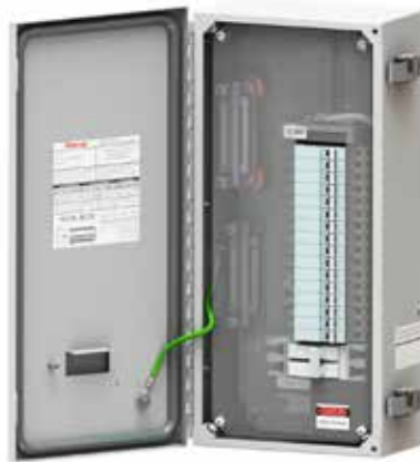
RSD-FMC-Z16MS-21NN (Lt. Gray color, 16 Breakers, Strikesorb SPD, External Disconnect)
