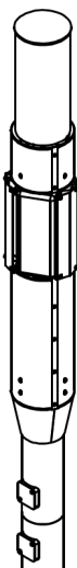
The top of the integrated small cell pole houses two 4G and three 5G radios.
