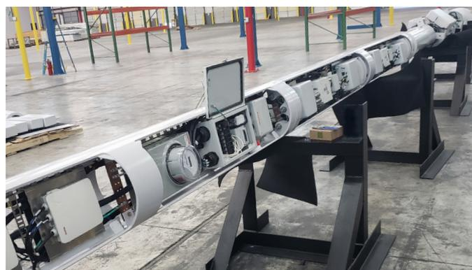
*Integrated small cell poles, like these at one of Raycap's three manufacturing facilities, contain and conceal complete small cell sites.*
